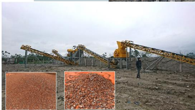
Recycled coarse aggregates (RCA) from crushed concrete of size 10-20mm (left), and 5-10mm (right)
