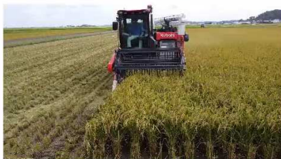
Self driving General purpose robot combine
